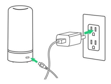
Your device comes partially charged so you can use it immediately. To fully charge your device, use the included charging cord. Please allow **4-6 hours** for a full charge. Always use the included wall charger to charge your AirMoji. Your device can be used as a portable unit once charged, or it can be used while plugged in.
