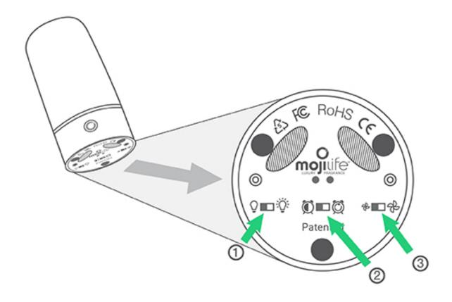
Once the AirMoji is powered on and in manual mode, you can control the LED light band, fan interval, and fan speed settings using the toggle switches located on the bottom of the device.
