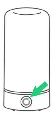
To turn off the AirMoji, press and hold power button for **3 seconds**. The power button light will turn off.
