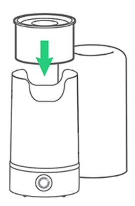
3. Insert pod (plastic cup with wood core) into the AirMoji.
