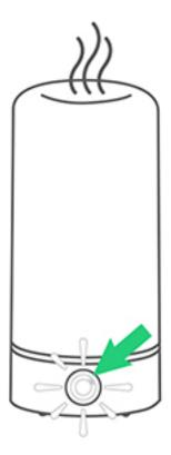
With your device in manual mode, press the power button again to enter **APP** mode. The light will then change from blue to white. Instructions for using the app to control the device can be found below.
